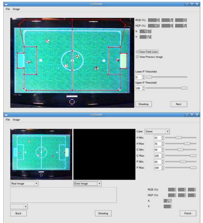
Fig. 2. The Calibrator program: calibrating field borders (up) and robot labels (down)
