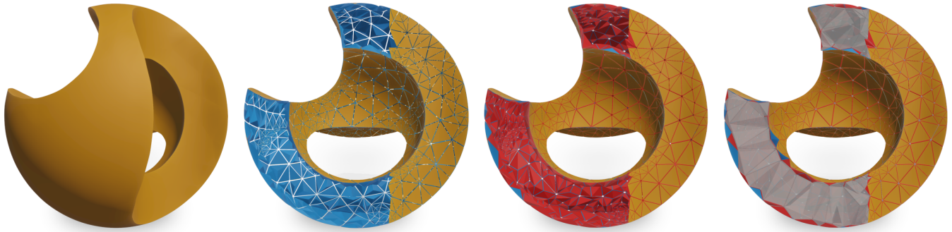
Fig. 18. Left: Input surface model Sculpture. Center: face and edge elements constructed for this. Right: Sliced view of the complete result mesh (including semi-transparent straight elements in gray).
